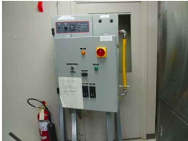
HyperFlo wash system with Total Control QuickPanel Jr. controller, control cabinet, wash tank, pump with HPS 30 kva transformer and Process Technologies TYTAN water heater TY-048-480-3
