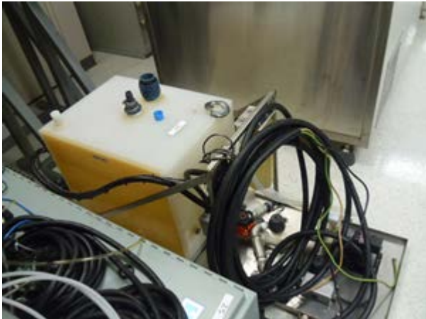
HyperFlo wash system with Total Control QuickPanel Jr. controller, control cabinet, wash tank, pump with HPS 30 kva transformer and Process Technologies TYTAN water heater TY-048-480-3
